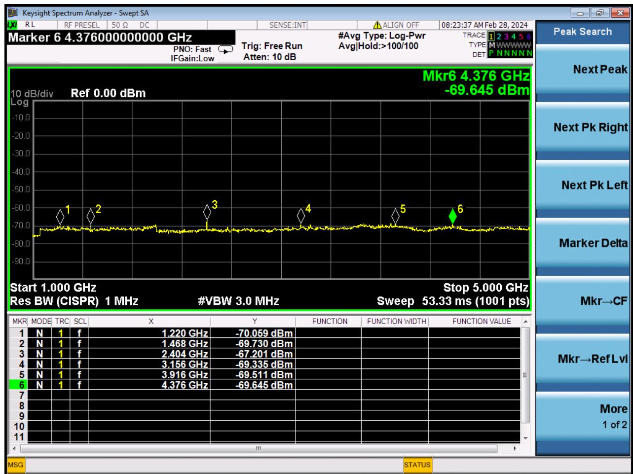
**V port, Operate at 930.5MHz, 30MHz -1000MHz**
