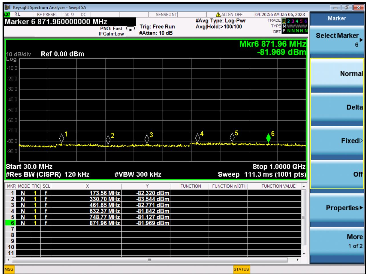
**V port, Operate at 901.5MHz, 1GHz -5GHz**
