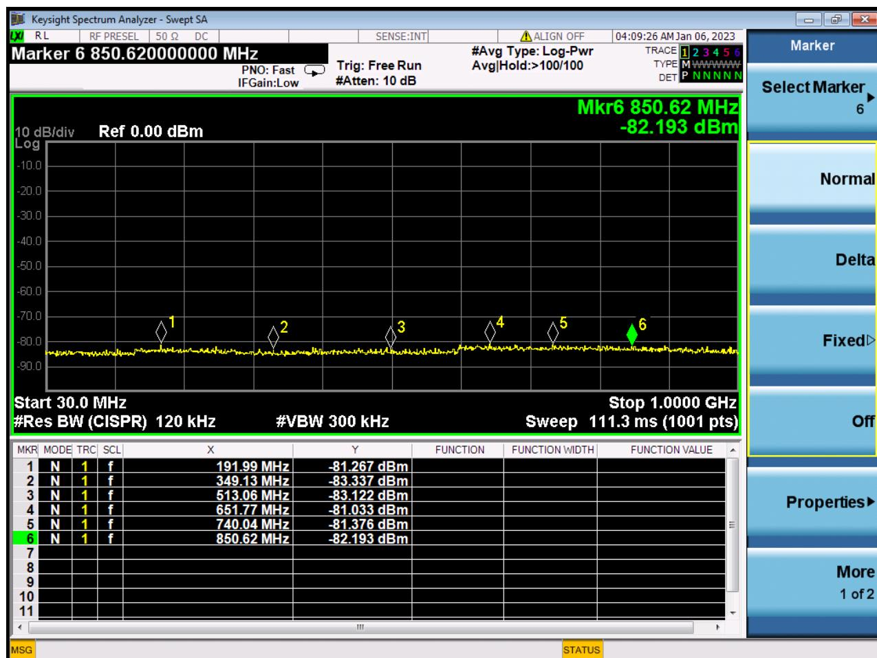
**H port, Operate at 901.5MHz, 1GHz -5GHz**
