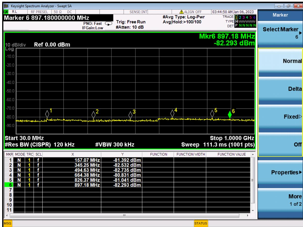
**V port, Operate at 930.5MHz, 1GHz -5GHz**
