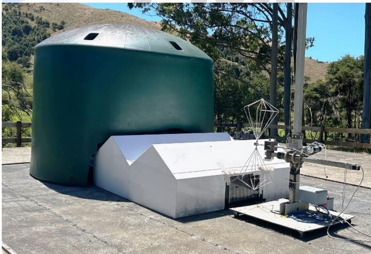
Biconical Antenna pointing towards Test Enclosure
