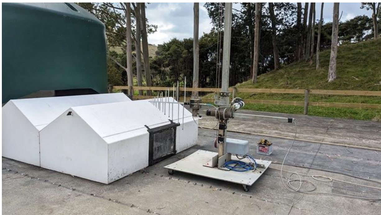
Log Periodic Antenna pointing towards Test Enclosure
