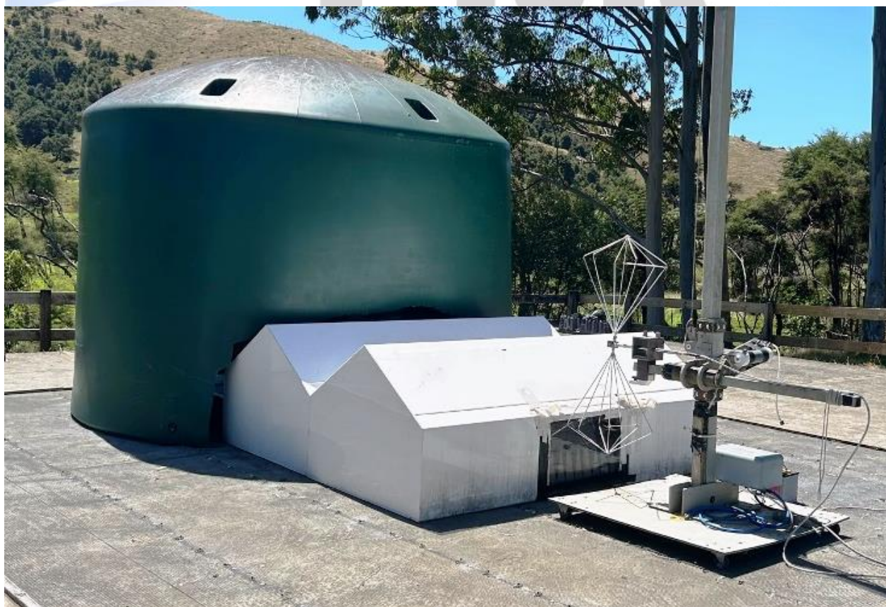
Biconical Antenna pointing towards Test Enclosure
