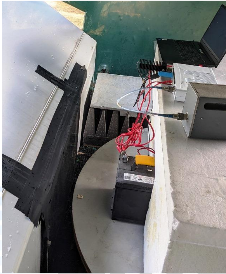
Biconical Antenna pointing towards Test Enclosure.
