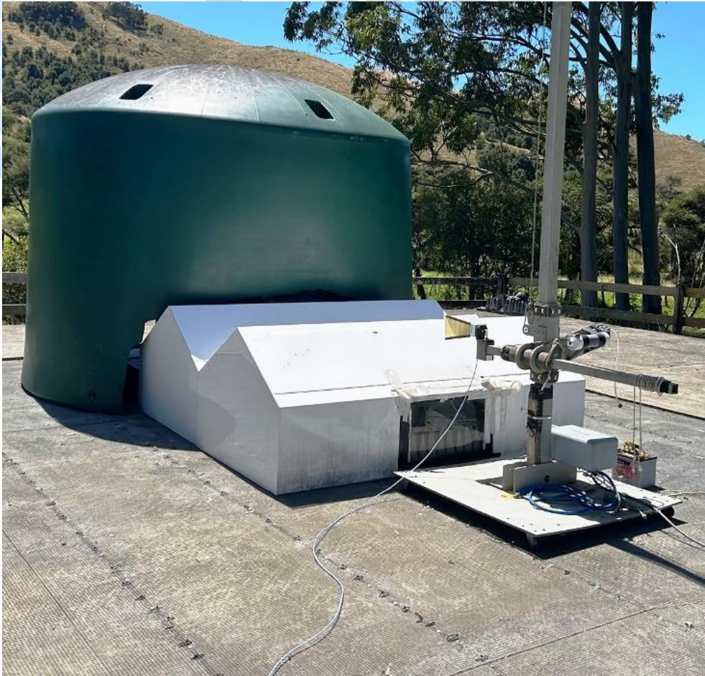
Horn Antenna pointing towards Test Enclosure.
