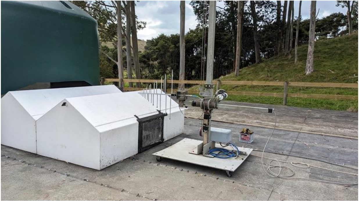
Horn Antenna pointing towards Test Enclosure.
