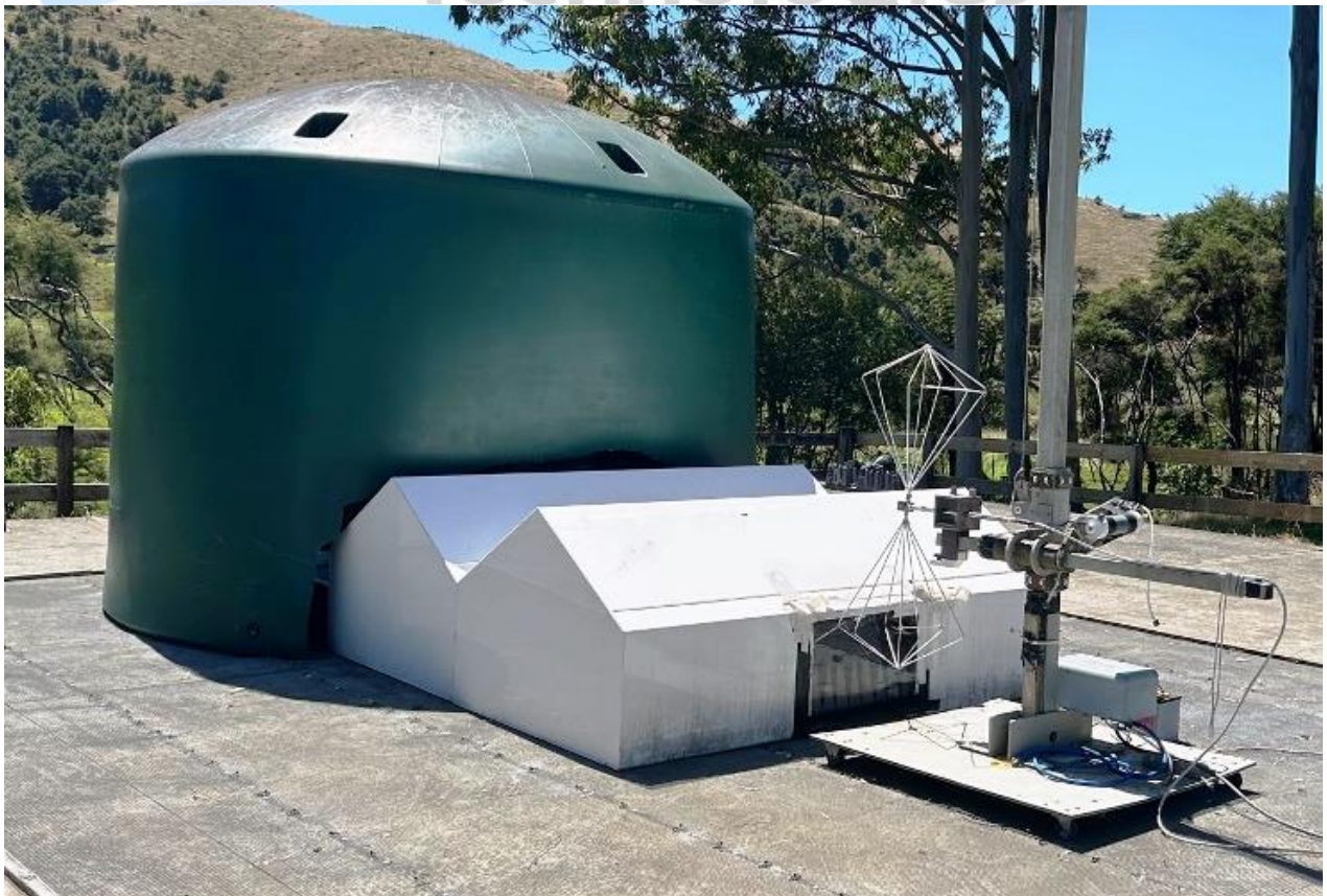
Biconical Antenna pointing towards Test Enclosure.
