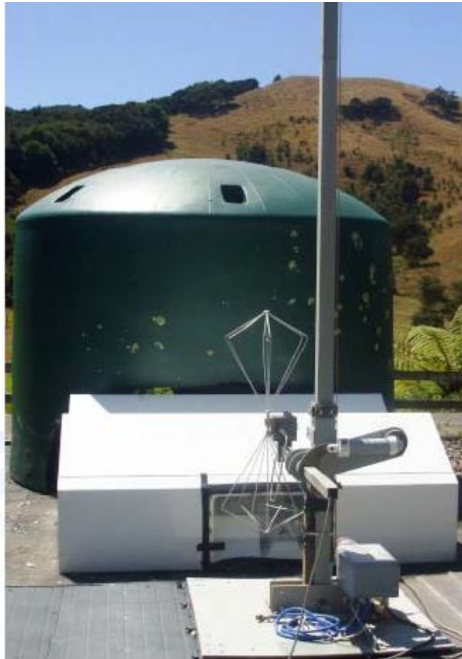
Test Shed showing the use of a Biconical Antenna
