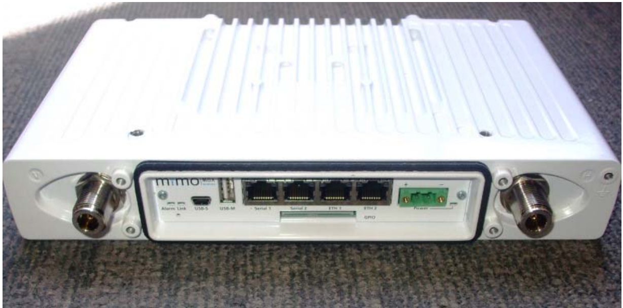
Face with antenna ports
