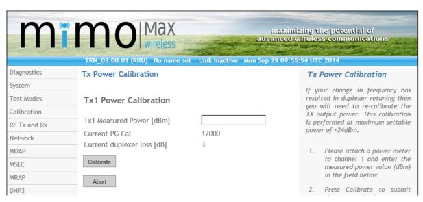
Figure 1: Tx Power Calibration
