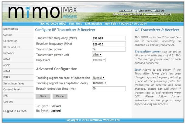
**Figure 2 Transmitter Power Setting**
