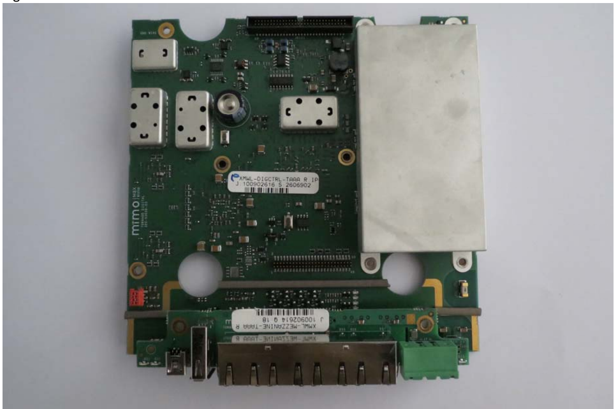
Digital mezzanine bottom with shields
