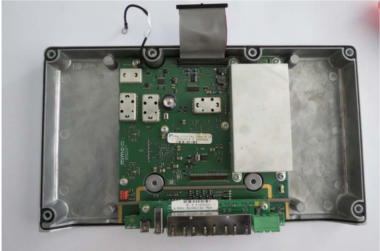
Digital mezzanine in chassis
