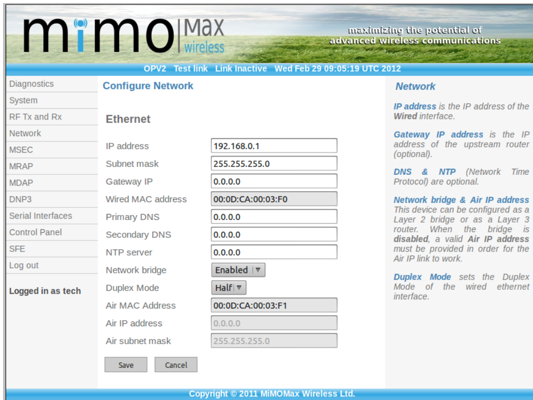
Figure 8- Network Configuration Page
