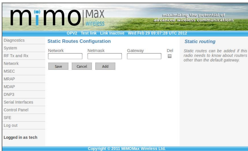
Figure 9 - Static Routing Page
