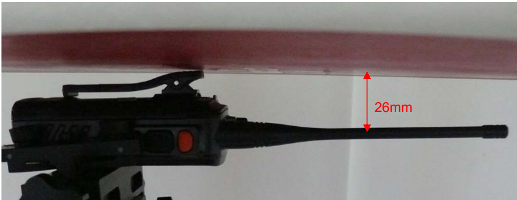
Picture 5: Body-worn, the front of the EUT towards ground, Belt clip directed tightly to touch the bottom of the flat phantom, the distance from the EUT Antenna to the bottom of the Phantom is 26mm
