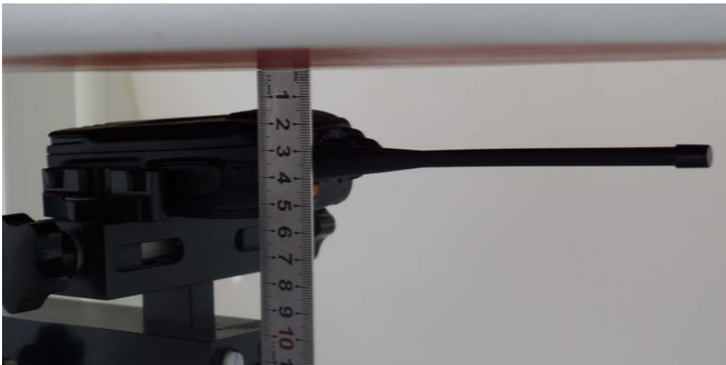
Picture 5: Body-worn, The EUT display towards ground, the distance from EUT to the bottom of the Phantom is 15mm
