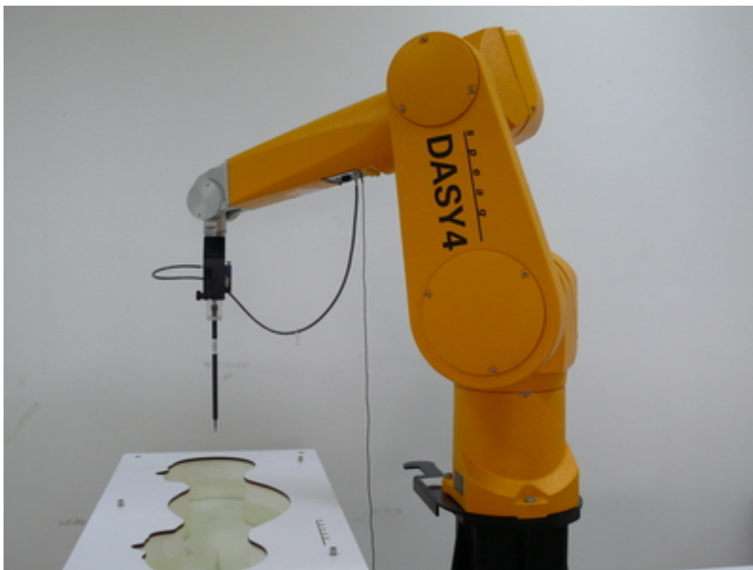
Picture 1: Specific Absorption Rate Test Layout
