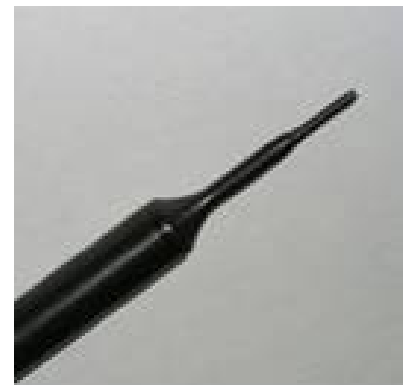
Figure 2. EX3DV4 E-field Probe
