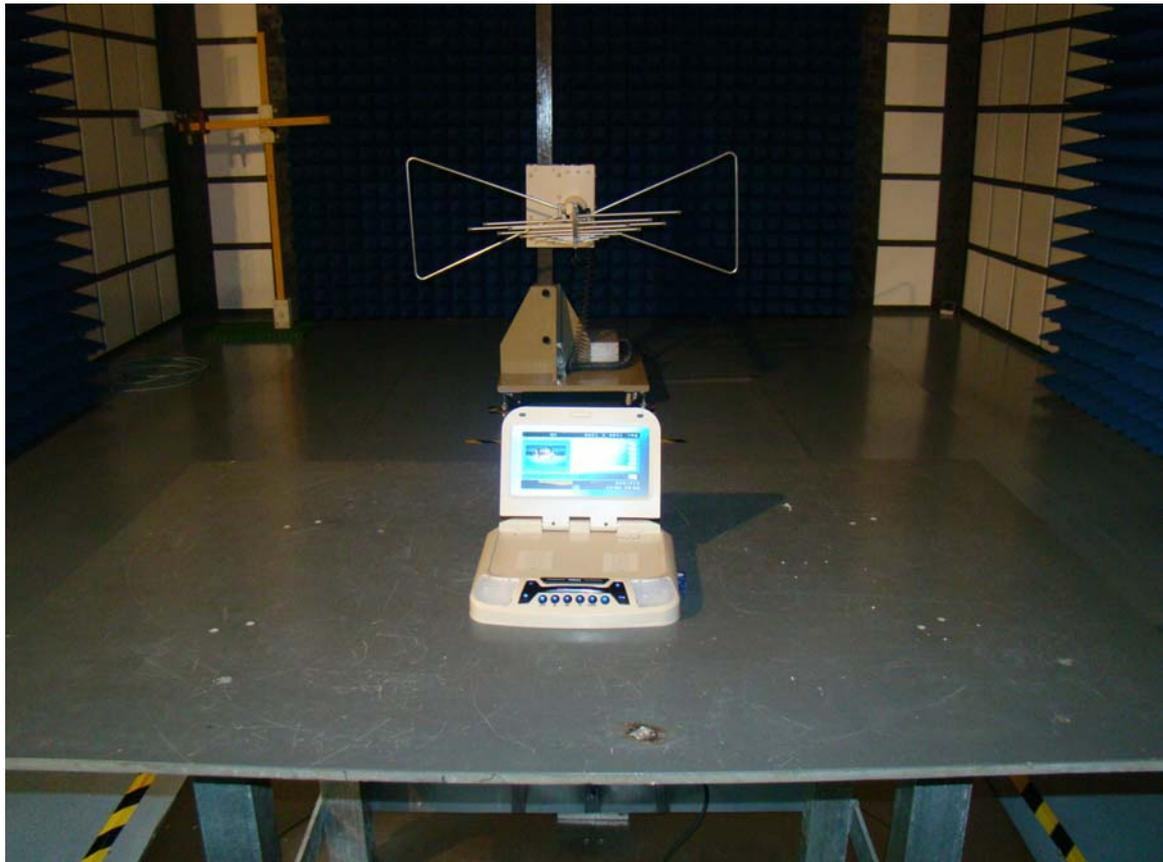
**Radiated emissions test: TX with Flash Disk**
