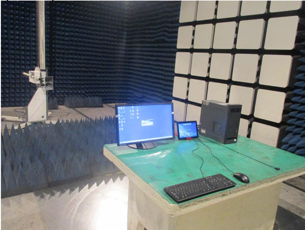
Photograph 3: Set-up for Radiated Emission of above 1GHz
