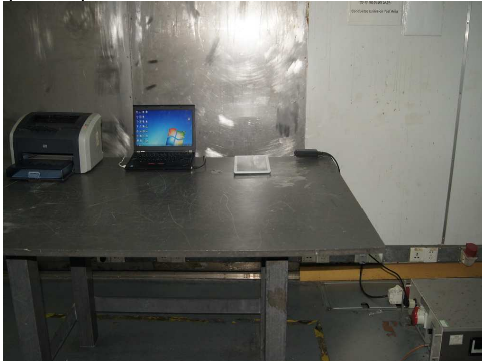
Photograph 2: Set-up for Spurious Emissions below 30MHz
