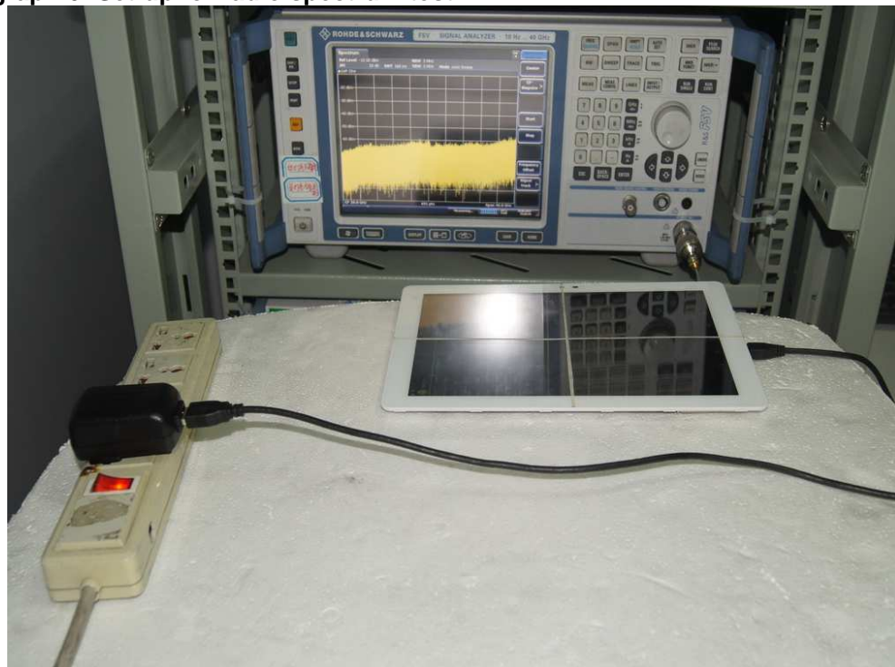
Photograph 6: Set-up for radio spectrum test
