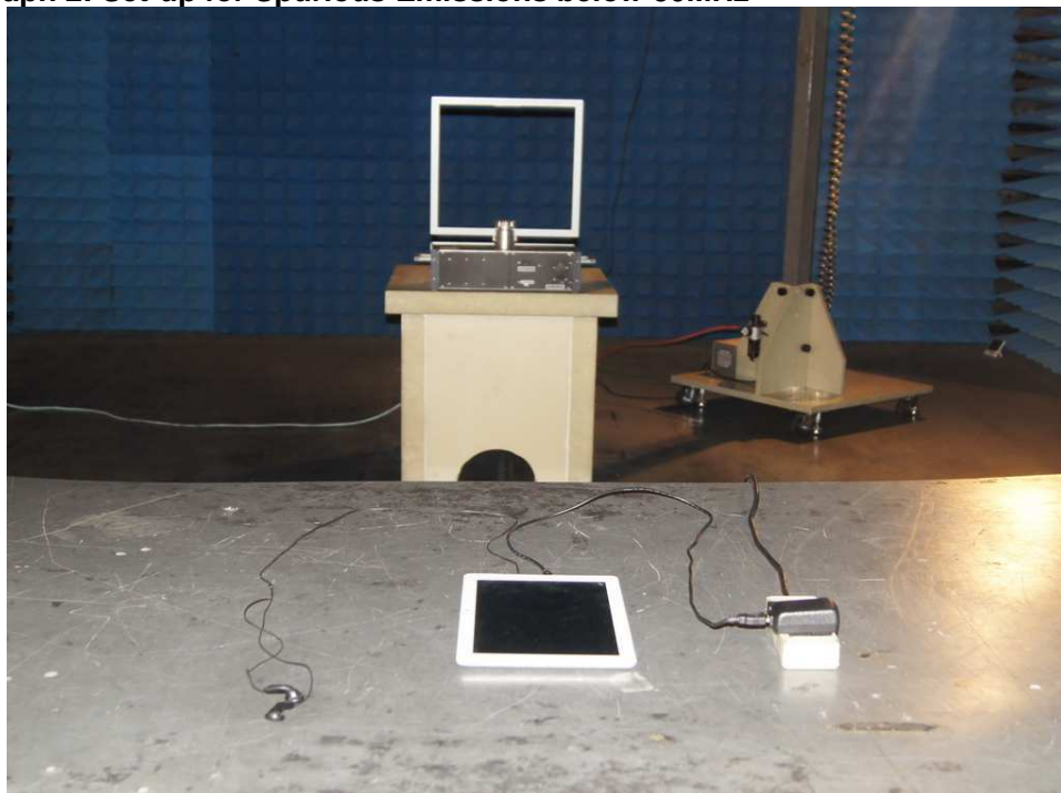
Photograph 2: Set-up for Spurious Emissions below 30MHz
