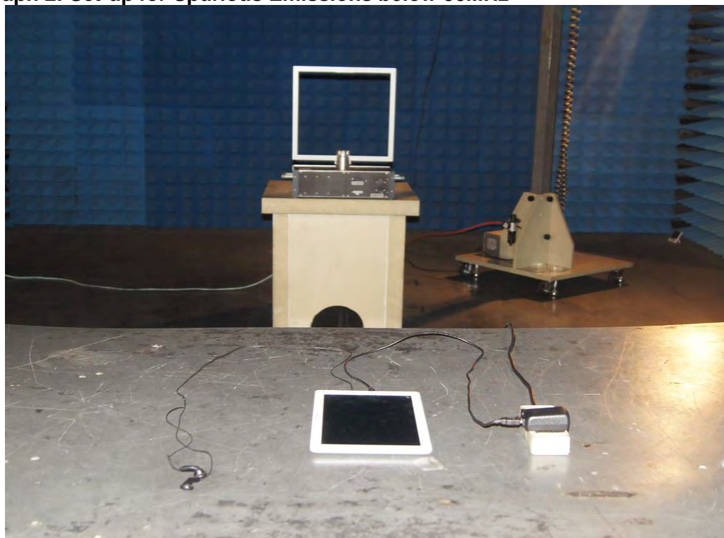
Photograph 2: Set-up for Spurious Emissions below 30MHz
