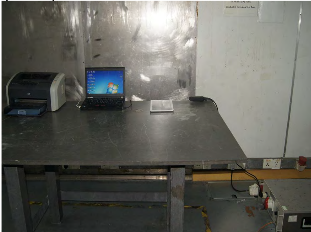
Photograph 2: Set-up for Spurious Emissions below 30MHz
