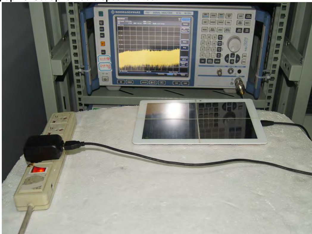
Photograph 6: Set-up for radio spectrum test
