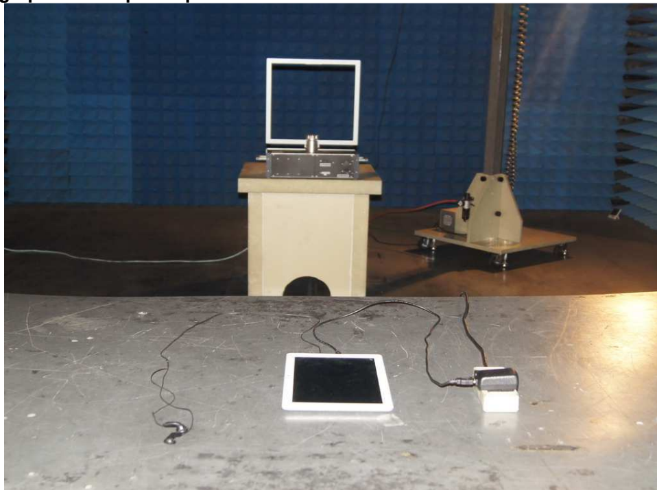
Photograph 2: Set-up for Spurious Emissions below 30MHz
