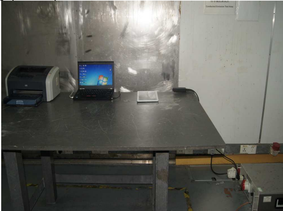
Photograph 2: Set-up for Spurious Emissions below 30MHz
