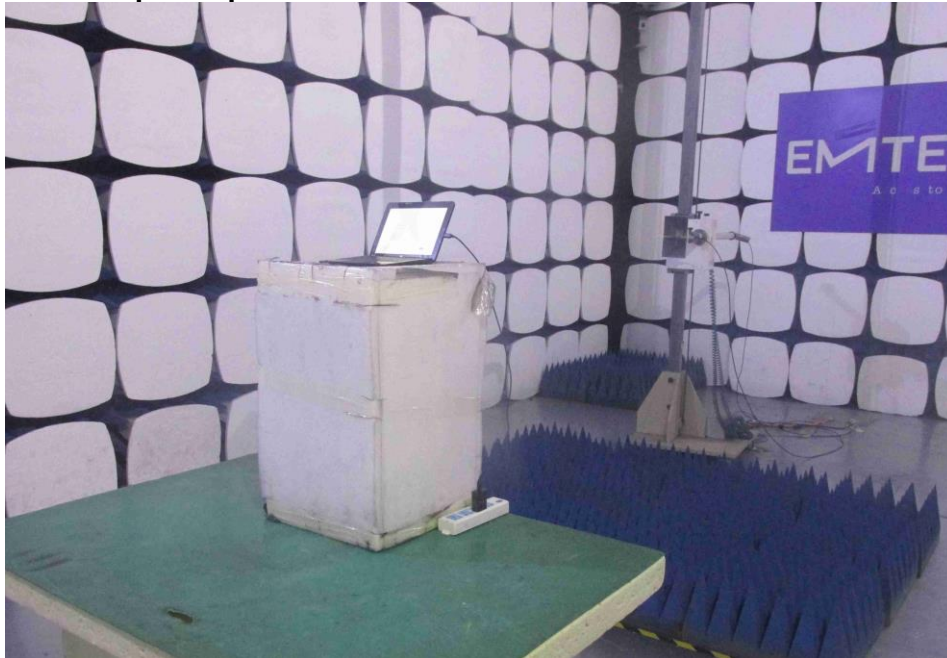
Photograph 4: Set-up for Spurious Emissions for 18 - 40GHz
