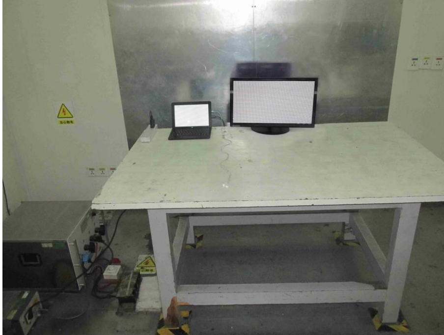
Photograph 2: Set-up for Spurious Emissions for 30 - 1000MHz
