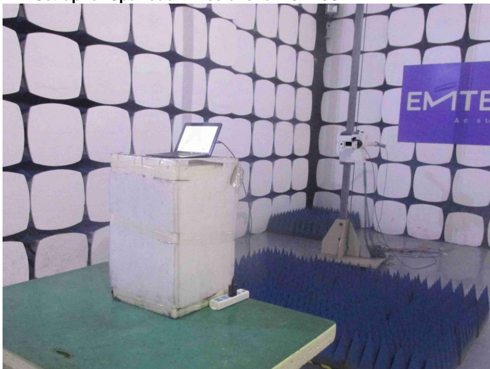
Photograph 4: Set-up for Spurious Emissions for 18 - 40GHz
