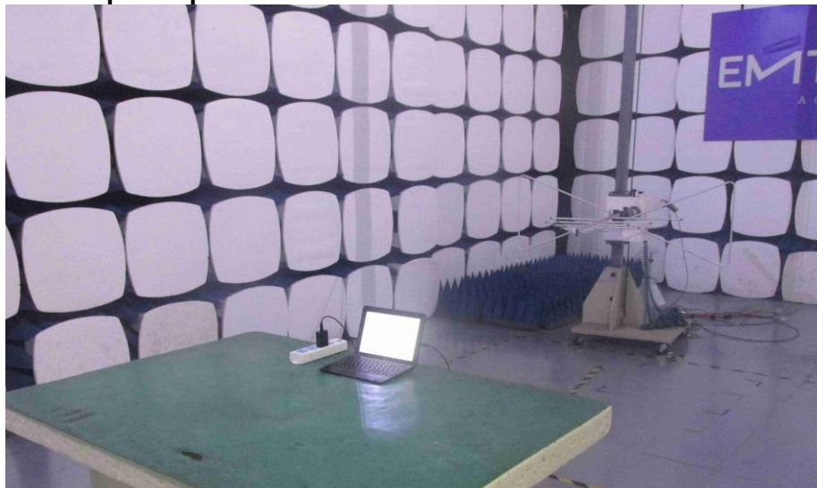
Photograph 2: Set-up for Spurious Emissions for 30 - 1000MHz
