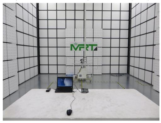
Description: Radiated Emission Test Setup for 1GHz ~ 18GHz (Mode 3)
