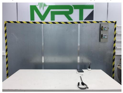
Description: Back view of Conducted Emission Test Setup (Mode 1, 2)
