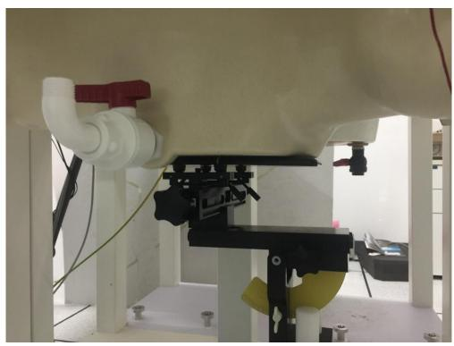
Description: 5G Wi-Fi SAR Test Photo (Worst case test setup "Back side")
