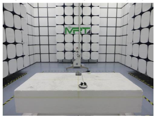
Description: Radiated Emission Test Setup for 1GHz ~ 18GHz (Mode 4)
