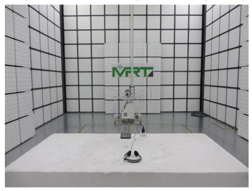
Description: Radiated Emission Test Setup for 1GHz  $\sim$  18GHz (Mode 1  $\sim$  2)
