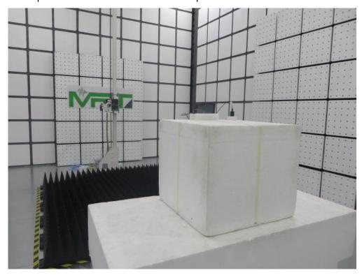
Description: Radiated Emission Test Setup for 18GHz ~ 25GHz
