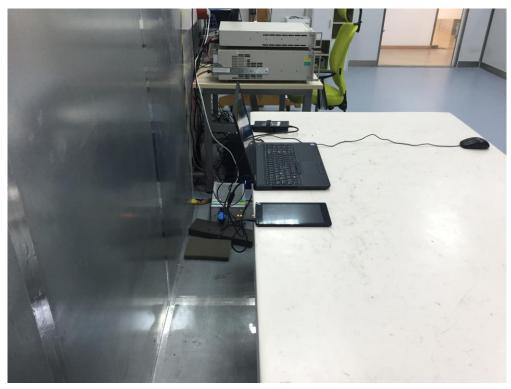
Description: Front view of Conducted Emission Test Setup (Mode 4)
