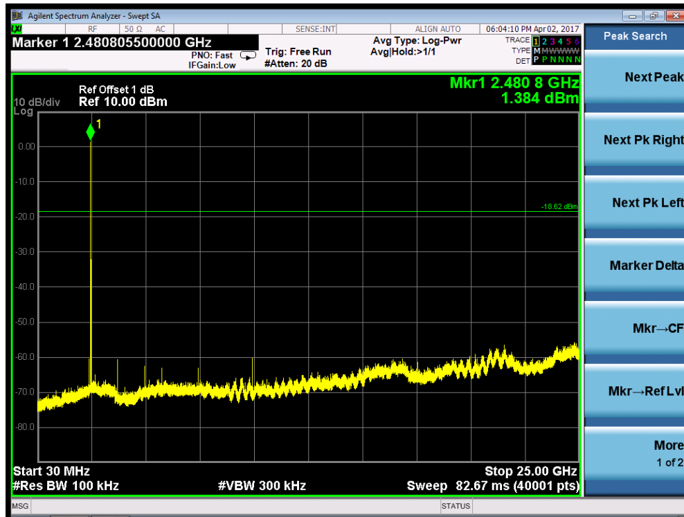
Figure 12: Conducted Spurious Emission, TM3
