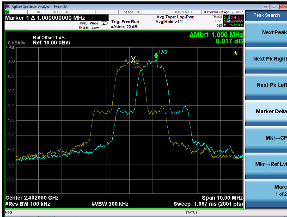
Figure 31: Frequency Separation, TM12, observation Frequency 2402MHz
