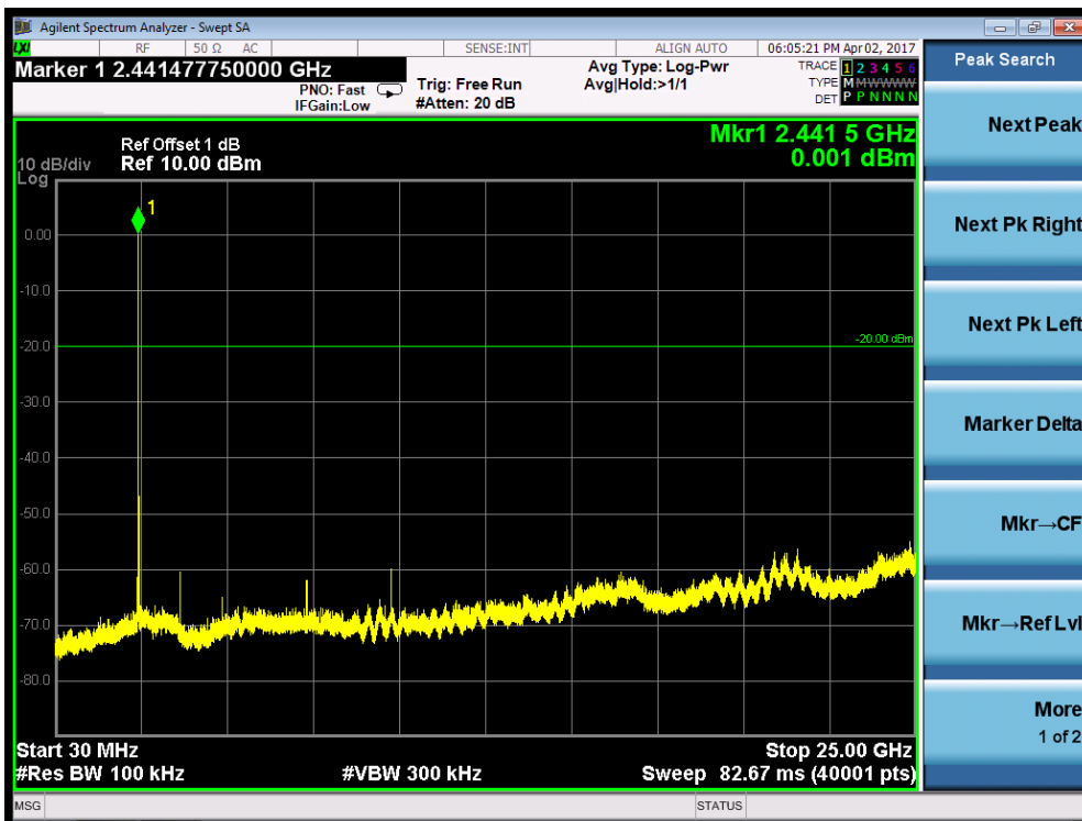
Figure 17: Conducted Spurious Emission, TM8
