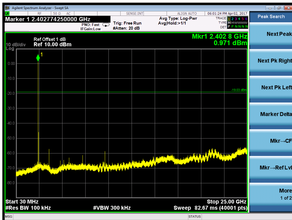
Figure 13: Conducted Spurious Emission, TM4
