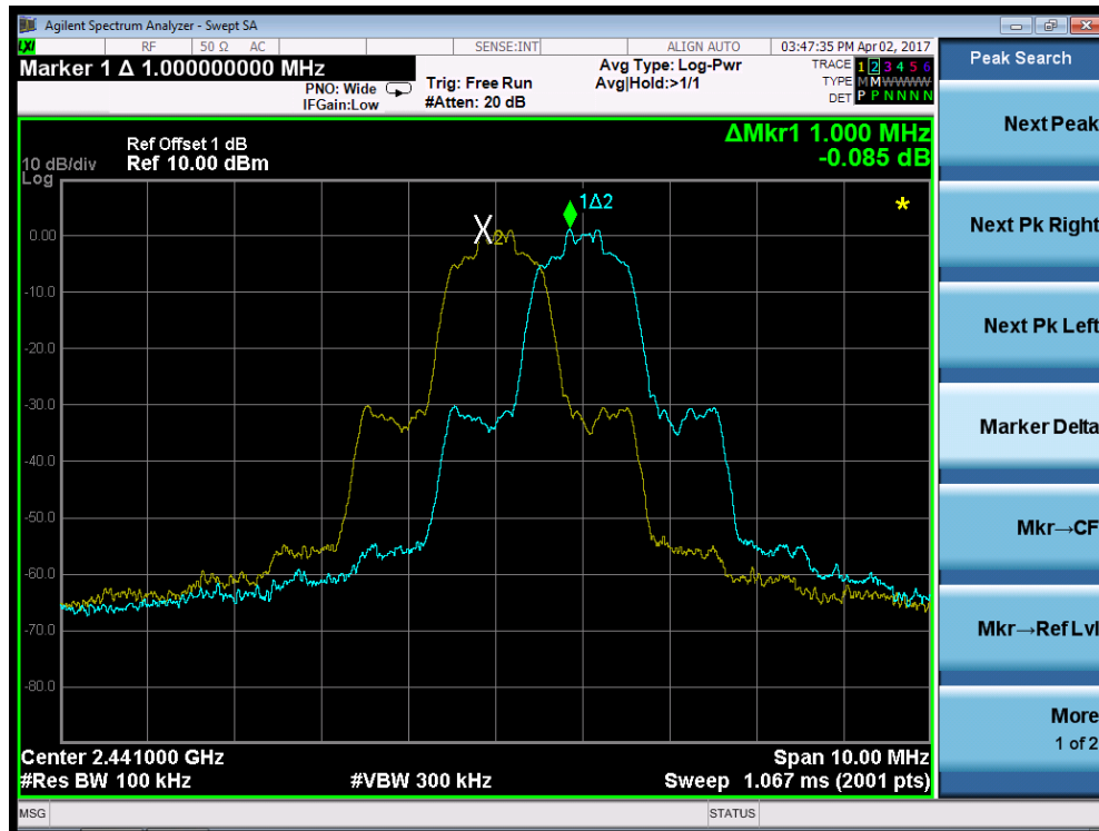
Figure 29: Frequency Separation, TM11, observation Frequency 2441MHz
