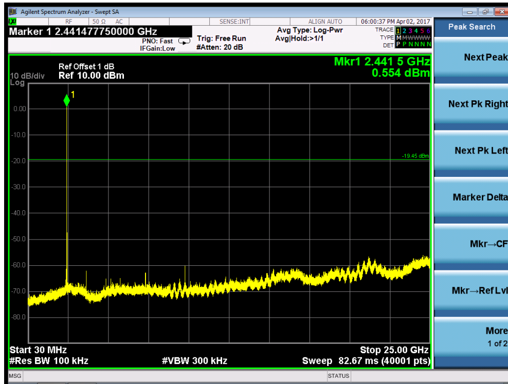
Figure 14: Conducted Spurious Emission, TM5
