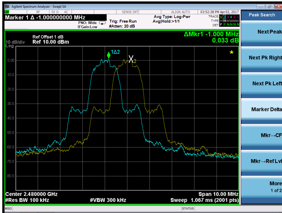
Figure 33: Frequency Separation, TM12, observation Frequency 2480MHz
