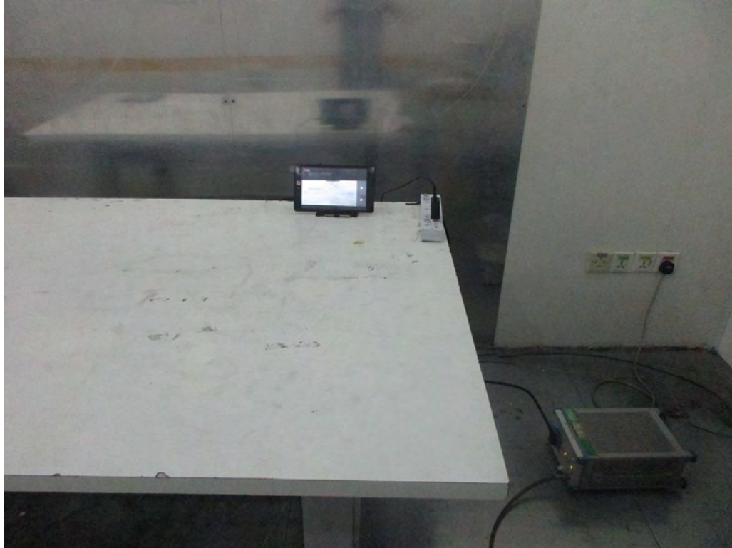
Photograph 2: Set-up for Spurious Emissions for below 30MHz
