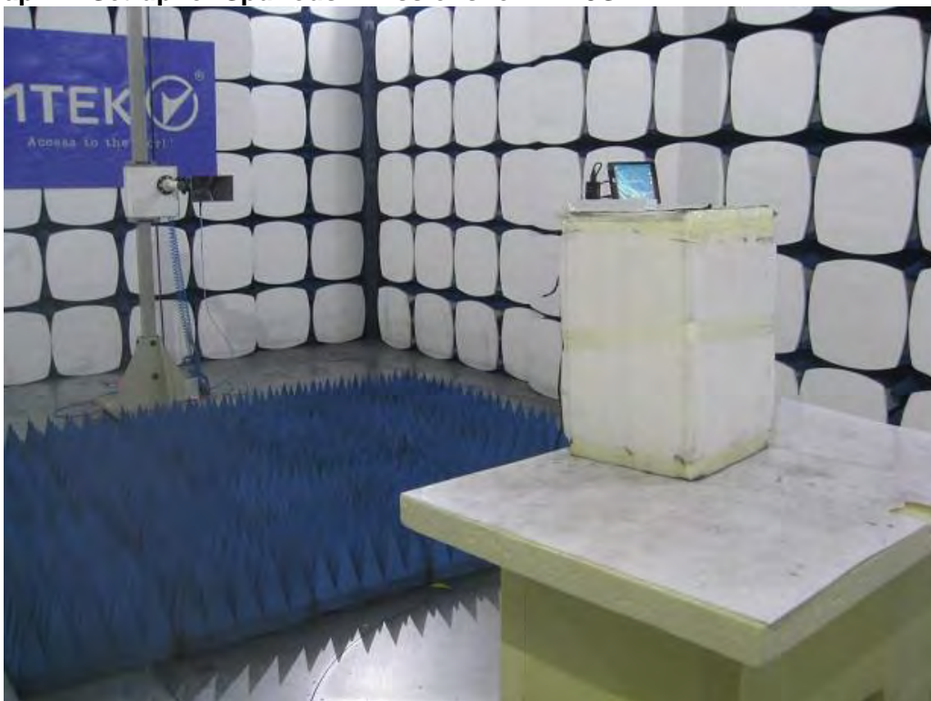
Photograph 4: Set-up for Spurious Emissions for 1 - 18GHz
