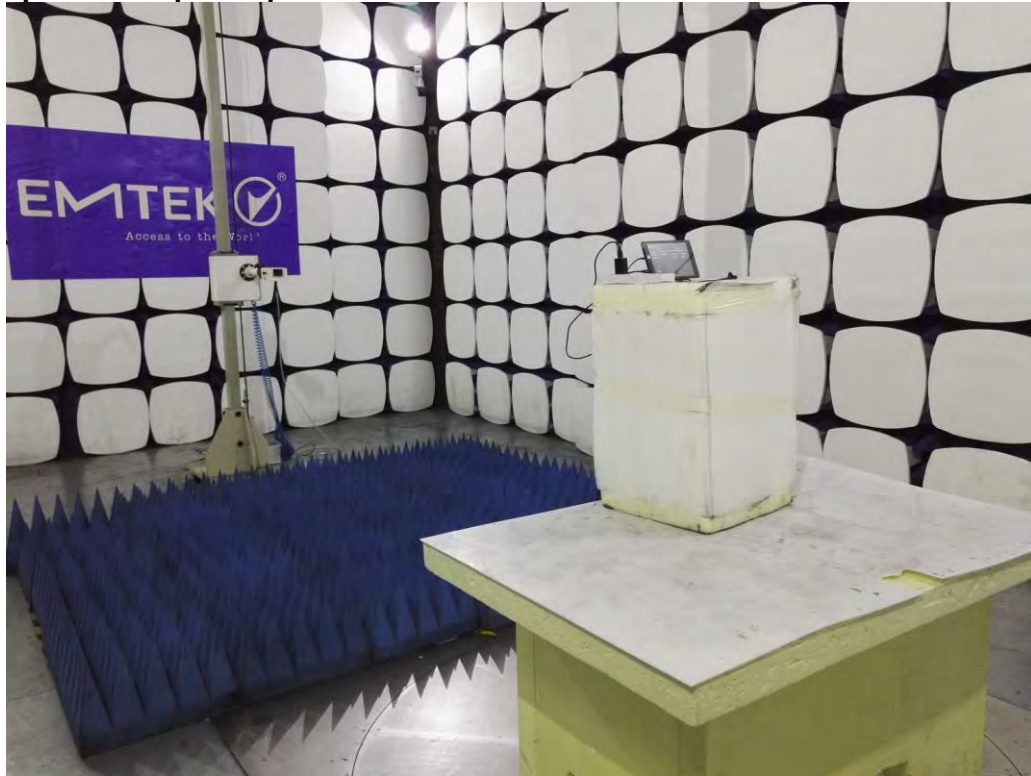
Photograph 5: Set-up for Spurious Emissions for 18 - 26.5GHz
