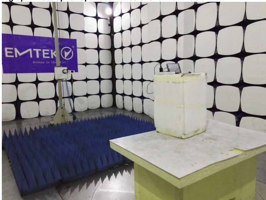
Photograph 4: Set-up for Spurious Emissions for 18 – 26.5GHz
