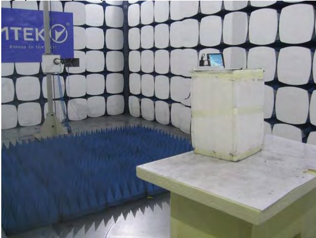
Photograph 4: Set-up for Spurious Emissions for 18 – 26.5GHz
