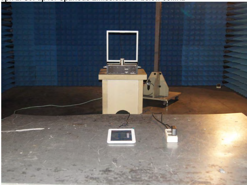
Photograph 2: Set-up for Spurious Emissions for below 30MHz
