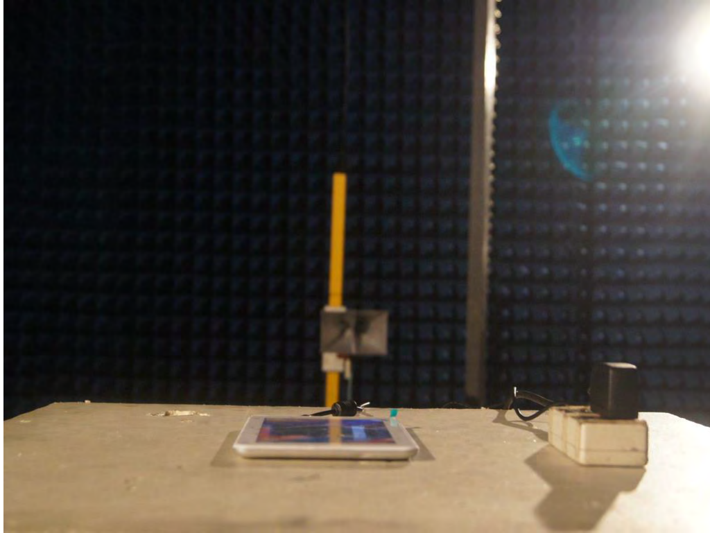
Photograph 6: Set-up for Spurious Emissions for 18 - 26.5GHz
