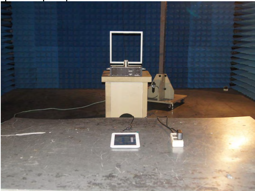
Photograph 2: Set-up for Spurious Emissions for below 30MHz
