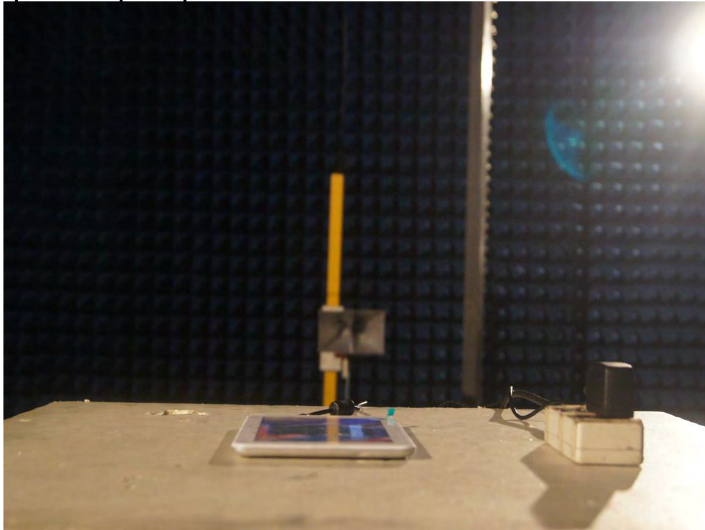
Photograph 6: Set-up for Spurious Emissions for 18 - 26.5GHz
