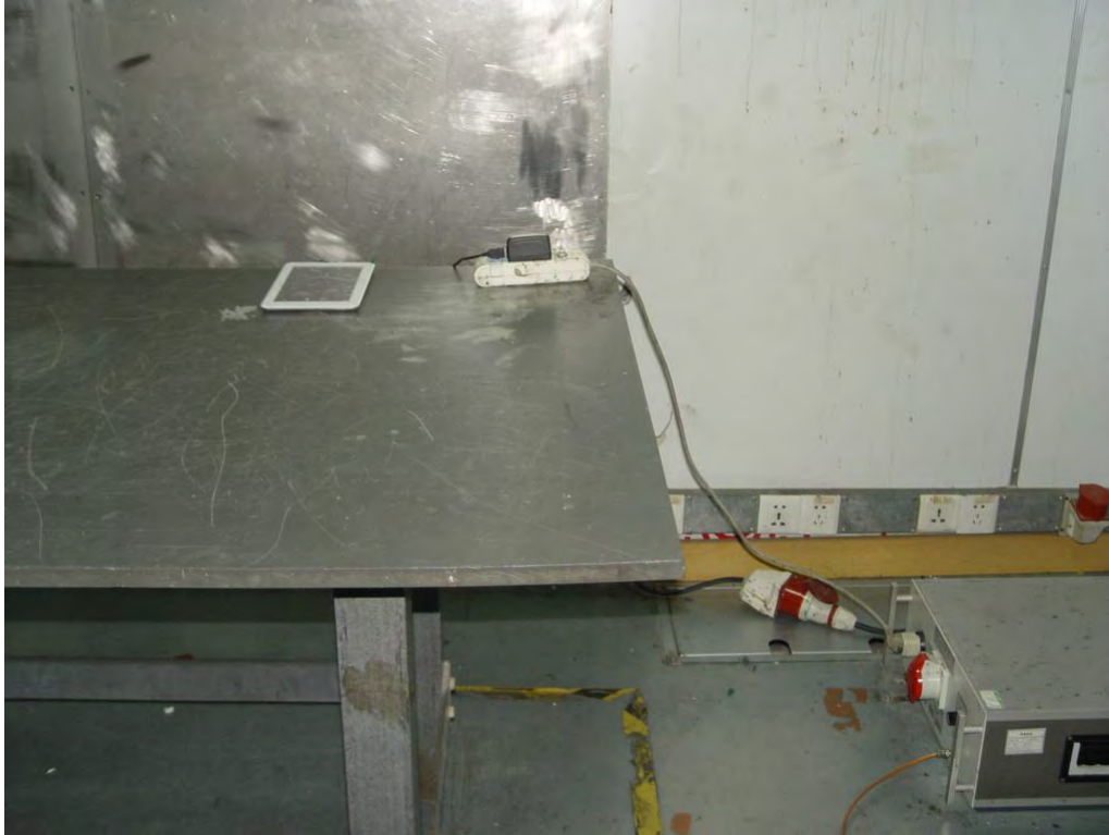
Photograph 2: Set-up for Spurious Emissions for below 30MHz
