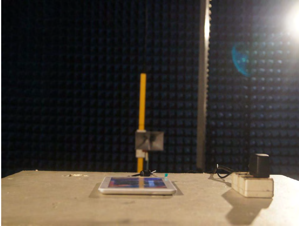
Photograph 6: Set-up for Spurious Emissions for 18 - 26.5GHz
