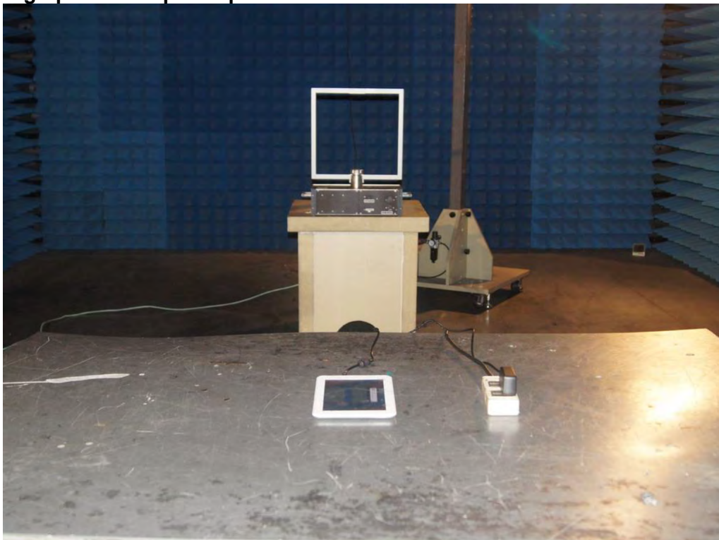
Photograph 2: Set-up for Spurious Emissions for below 30MHz
