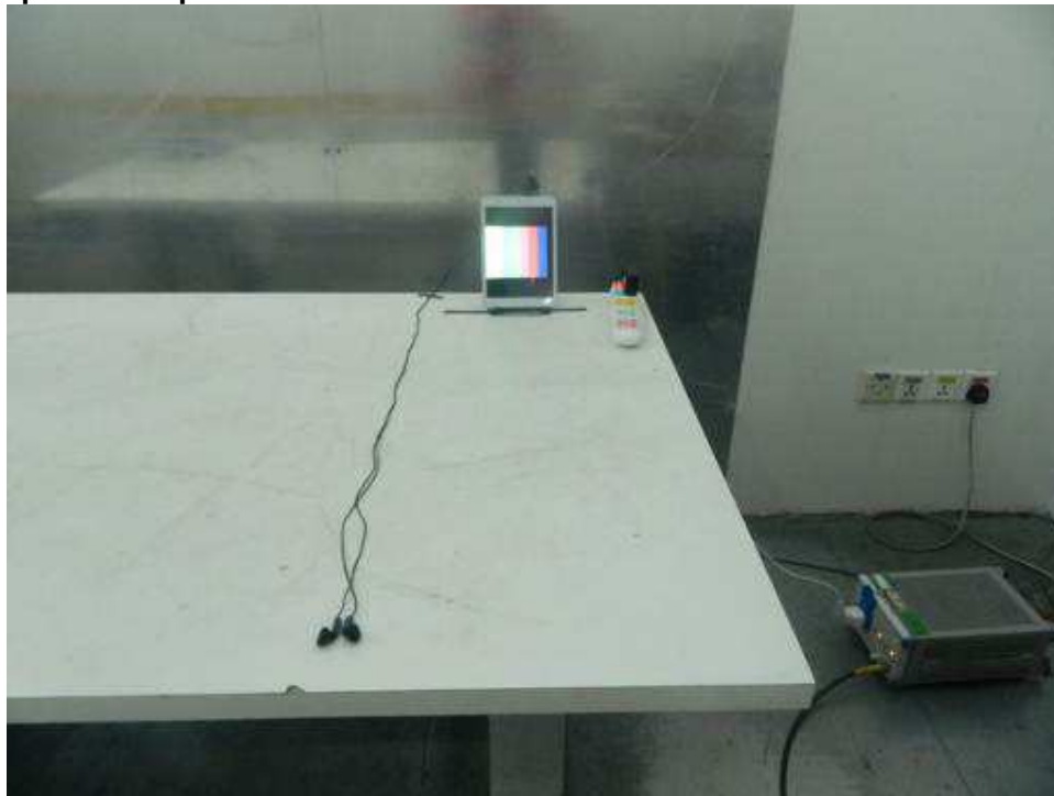
Photograph 1: Set-up for Conducted Emissions
