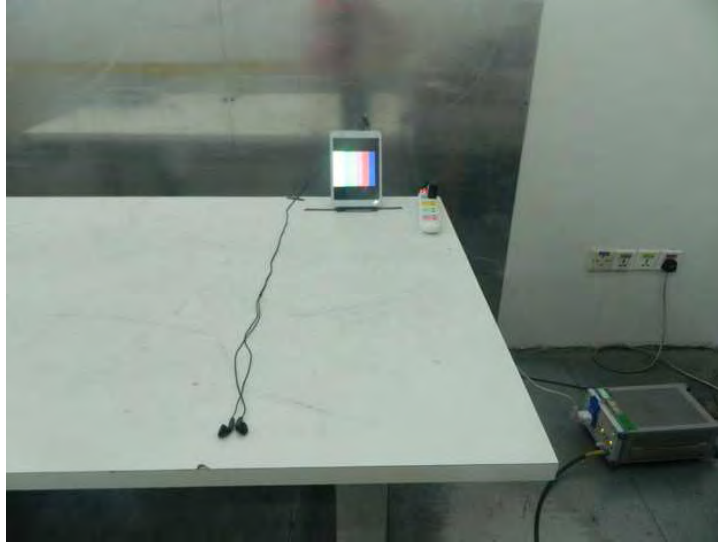
Photograph 1: Set-up for Conducted Emissions
