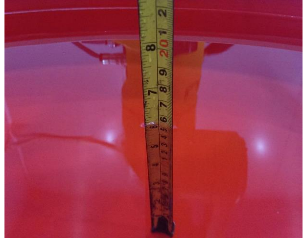
Photograph 2: Liquid Depth in the flat phantom (2450MHz, 15.5cm)
