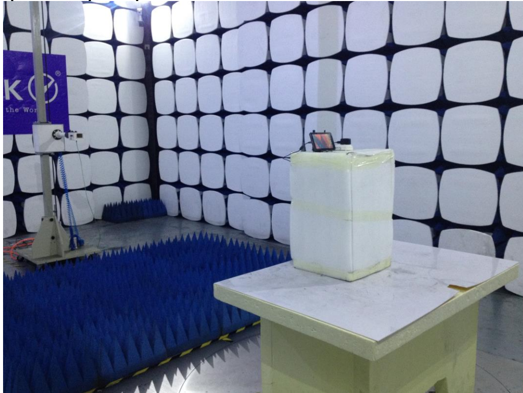
Photograph 5: Set-up for Spurious Emissions for 18 - 40GHz
