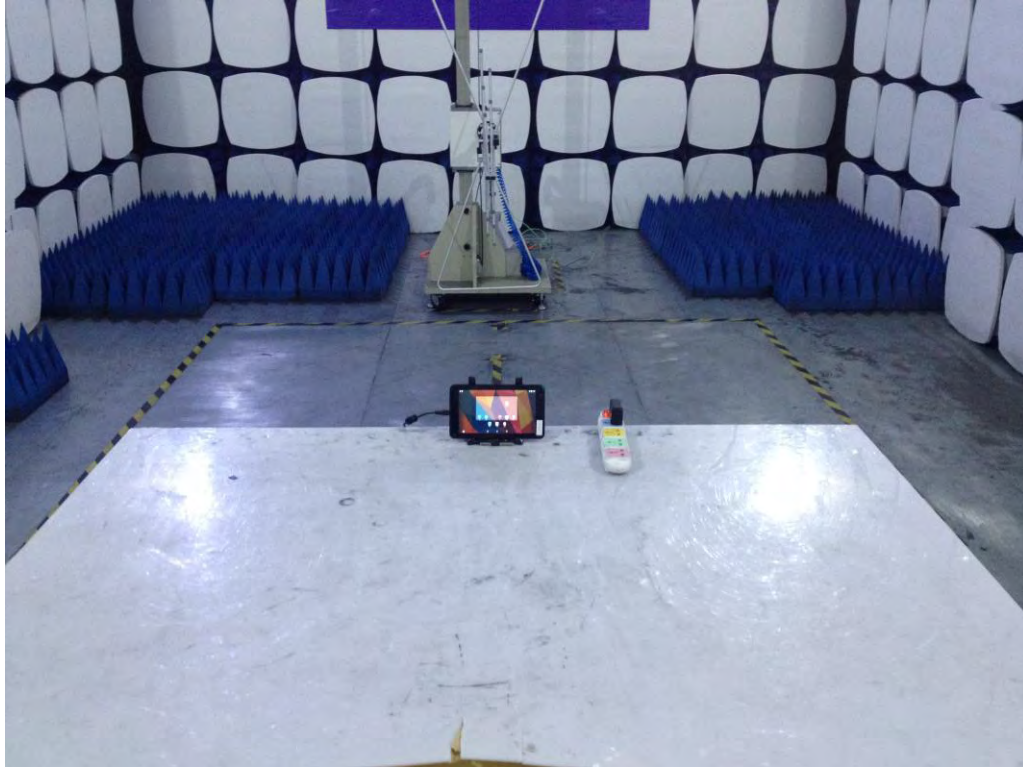
Photograph 4: Set-up for Spurious Emissions for 1 - 18GHz
