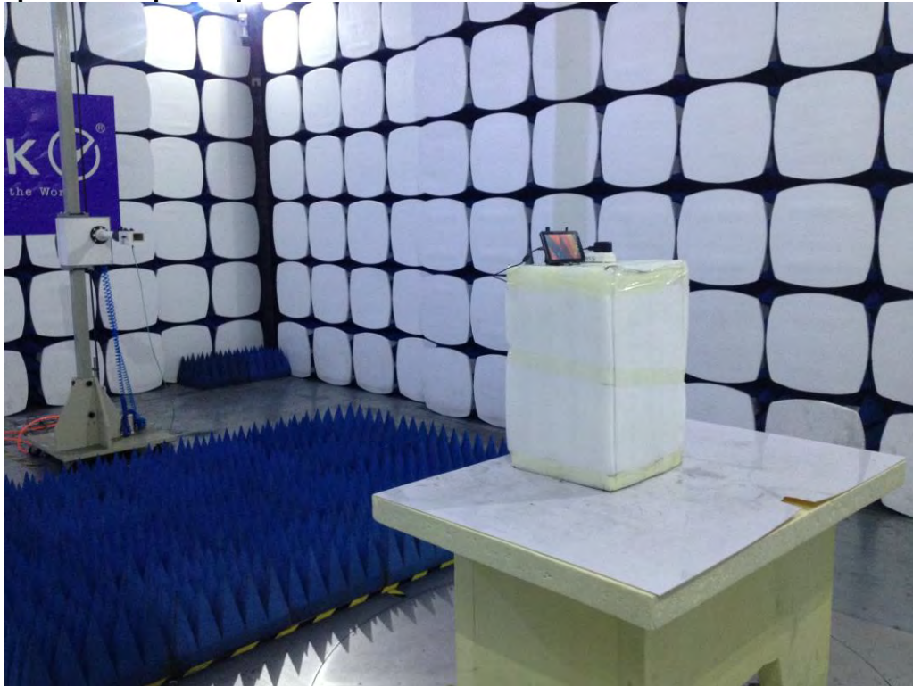
Photograph 5: Set-up for Spurious Emissions for 18 - 26.5GHz
