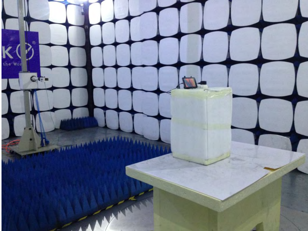
Photograph 5: Set-up for Spurious Emissions for 18 - 40GHz
