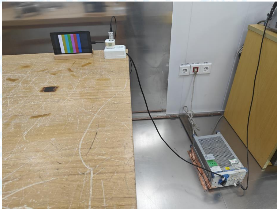
Photo of Setup for Conducted Emission
