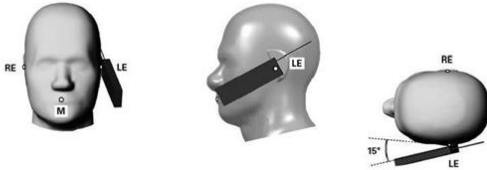
Picture16 Tilt position. The reference points for the right ear (RE), left ear (LE), and mouth (M), which define the Reference Plane for handset positioning, are indicated.
