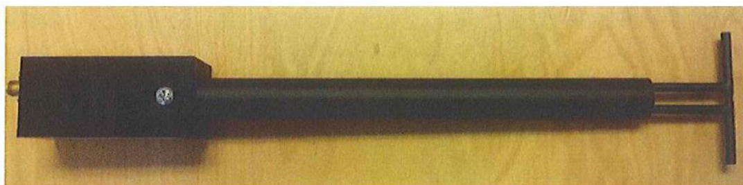
Figure 1 – MVG COMOSAR Validation Dipole
