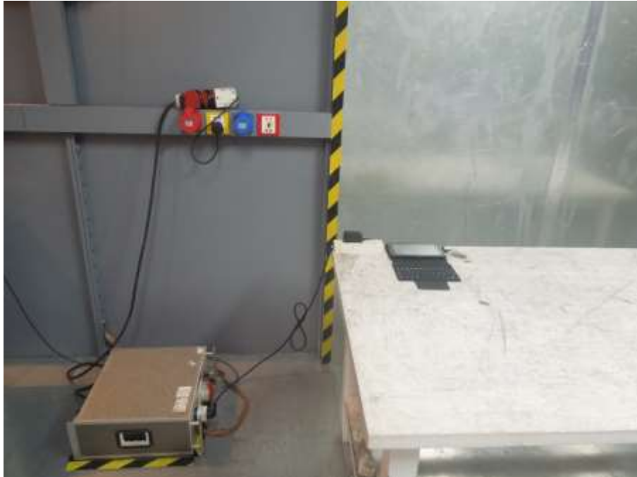
Photograph 3: Set-up for Conducted Emission on AC Mains
