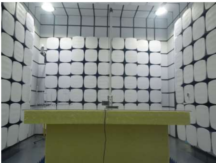
Photograph 2: Set-up for Radiated Spurious Emission (Above 1GHz)
