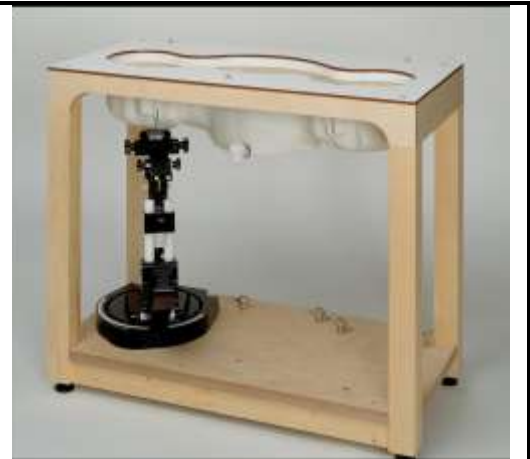
Fig. 8.7 Photo of SAM Twin Phantom
