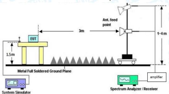
**Above 1GHz Test Setup**
