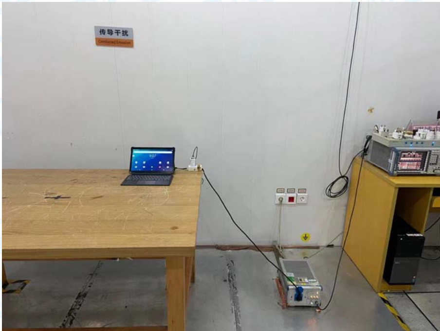
Photo of Setup for Conducted Emission
