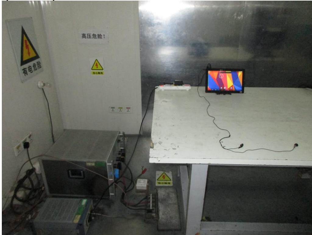
Photograph 2: Set-up for Spurious Emissions for below 30MHz
