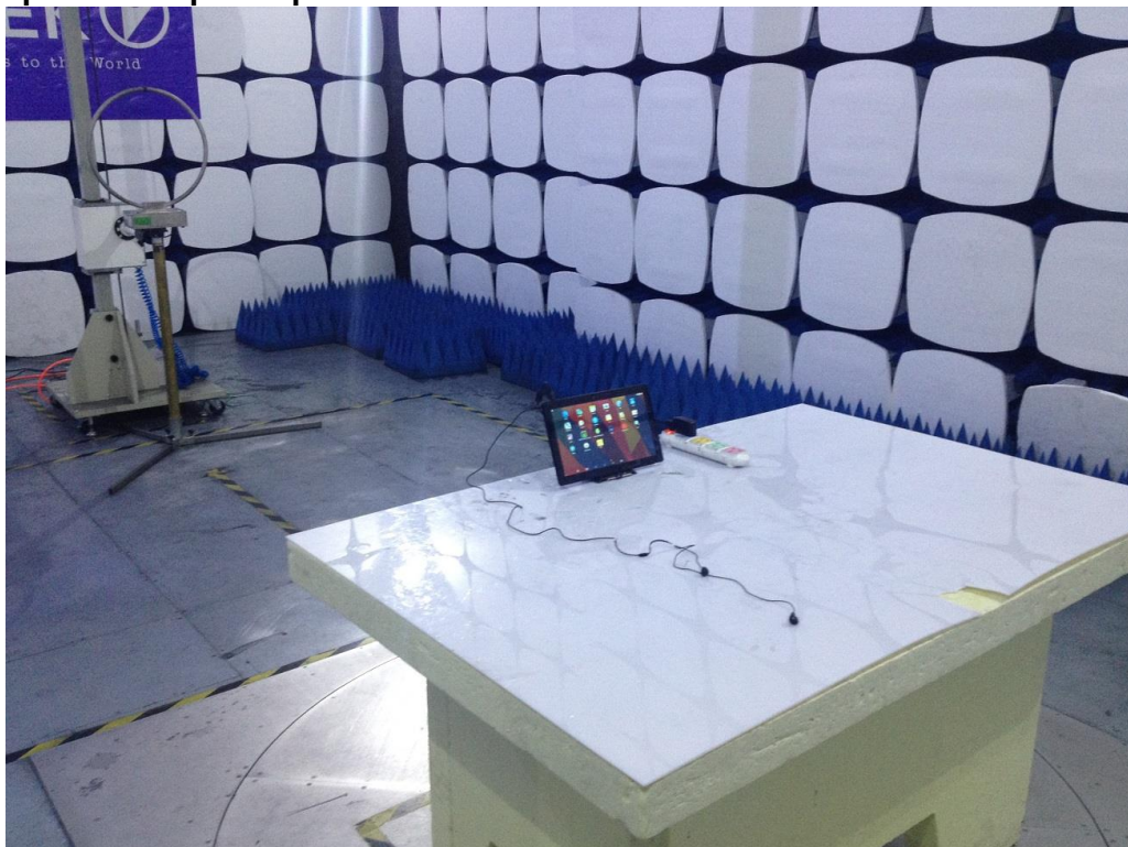
Photograph 2: Set-up for Spurious Emissions for below 30MHz
