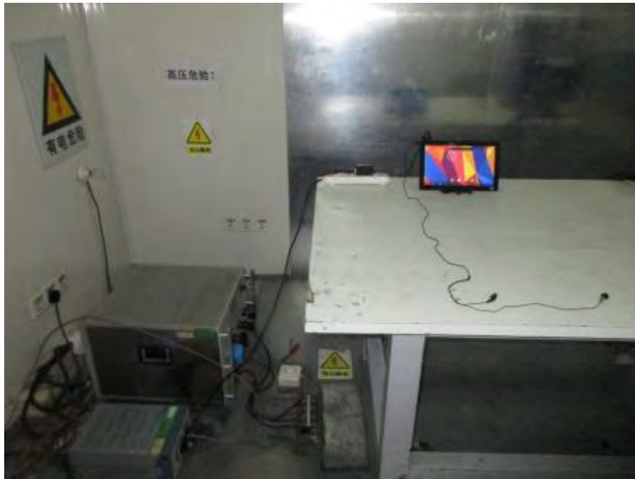
Photograph 5: Set-up for Conducted Emission
