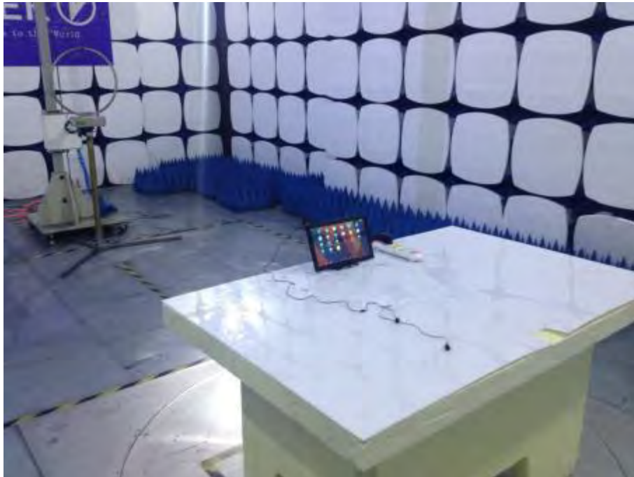
Photograph 2: Set-up for Radiated Spurious Emission (30MHz ~ 1GHz)
