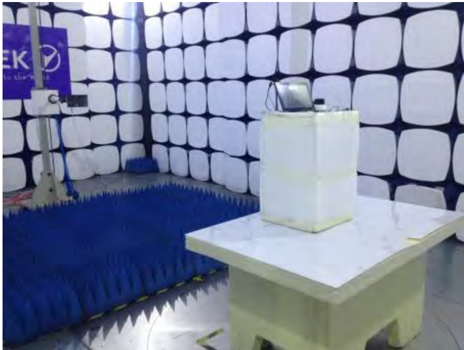
Photograph 4: Set-up for Radiated Spurious Emission (18GHz ~ 26GHz)
