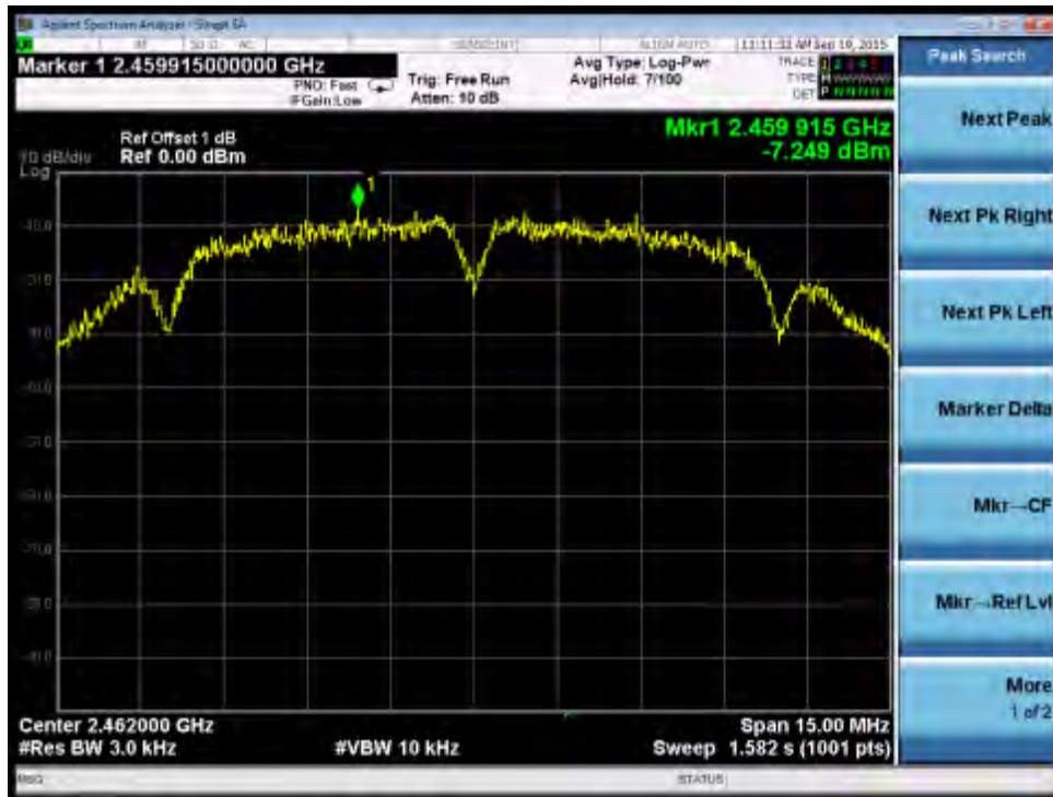
Test Plot of Power Spectral Density, 802.11g
