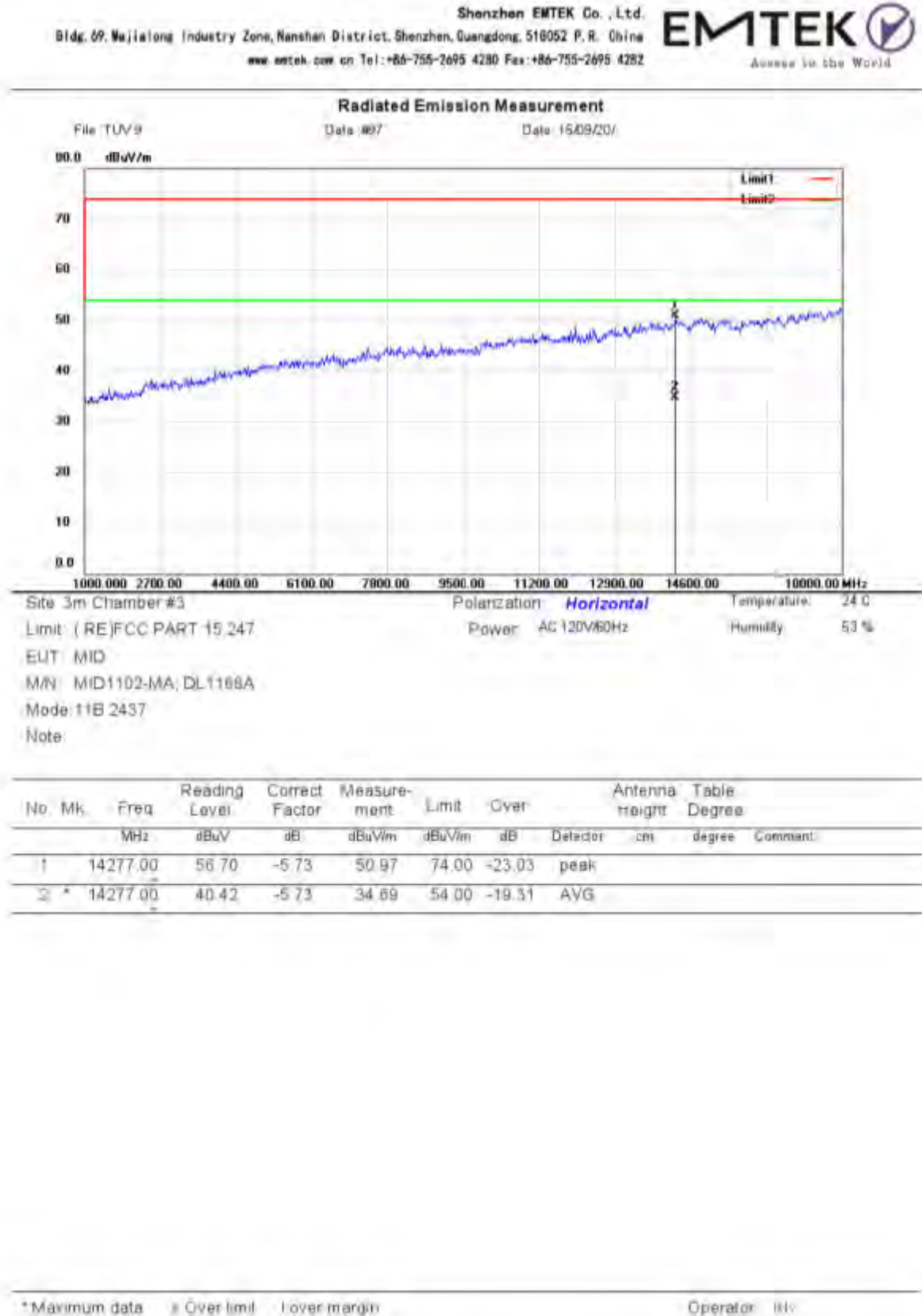
Figure 6: Test figure of Radiated Spurious Emissions (1GHz –25GHz), 802.11b, (Mid)
