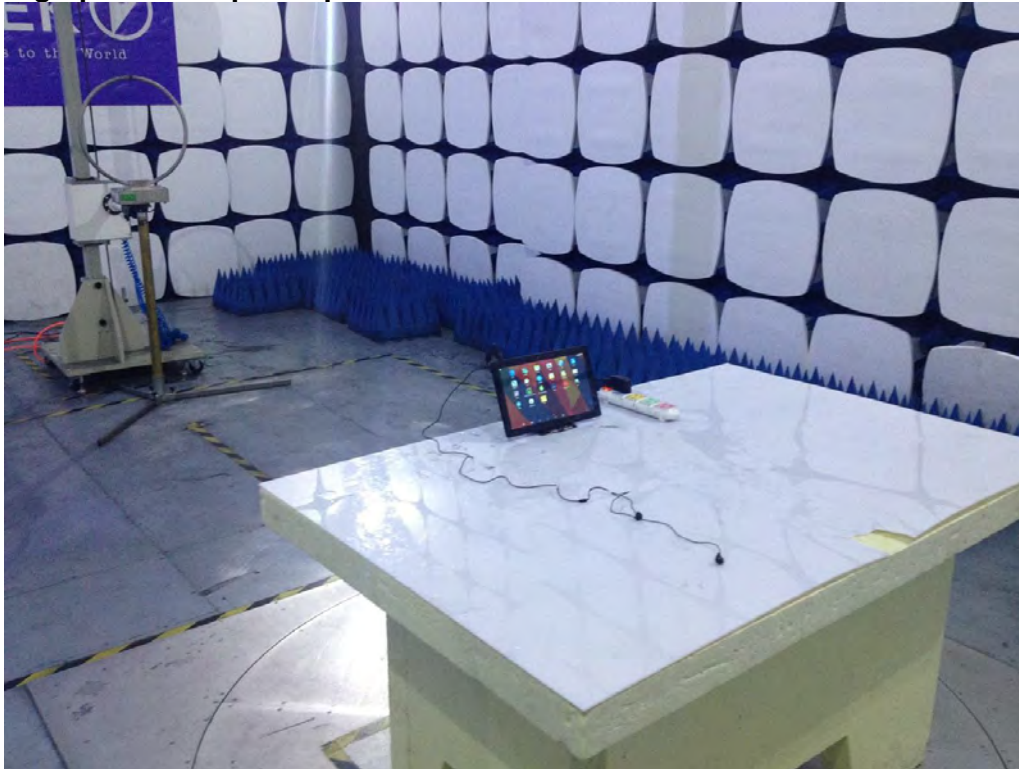
Photograph 2: Set-up for Spurious Emissions for 30 - 1000MHz
