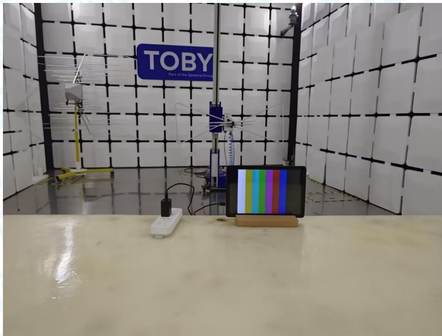
Photo of Setup for Radiated Emission (30MHz~1GHz)
