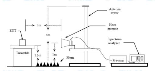
Above 1GHz Test Setup
