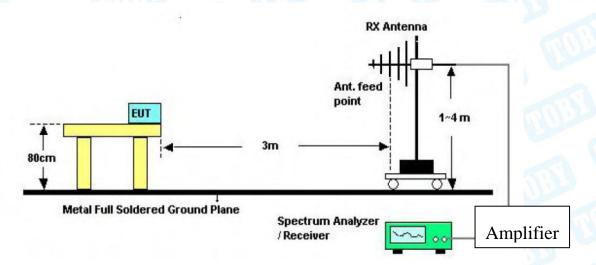
Below 1000MHz Test Setup
