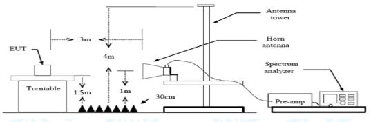
Above 1GHz Test Setup
