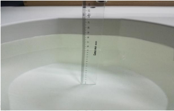
The Body Liquid of 2450MHz (15.3cm)
