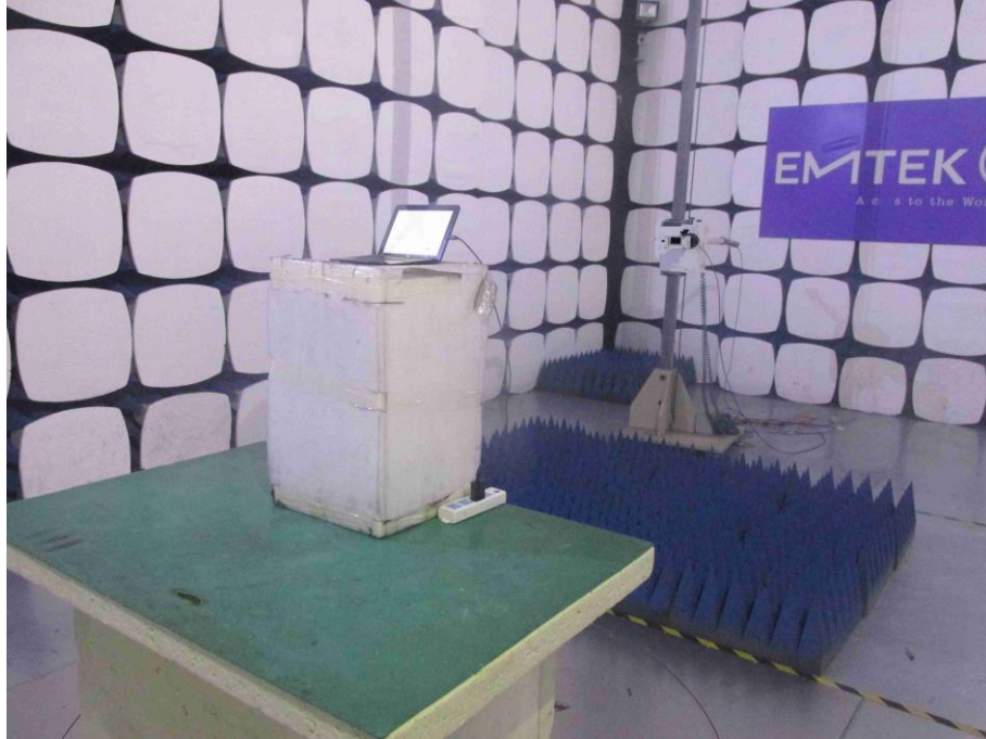
Photograph 4: Set-up for Conducted Emissions
