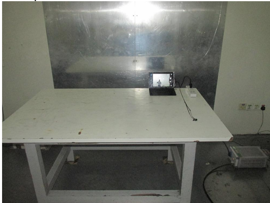
Photograph 4: Set-up for Conducted Emissions
