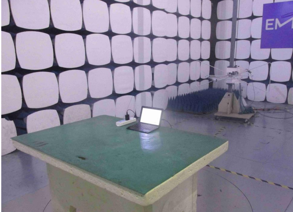
Photograph 2: Set-up for Spurious Emissions for 1 - 18GHz
