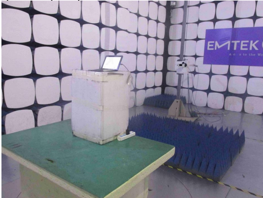
Photograph 4: Set-up for Conducted Emissions
