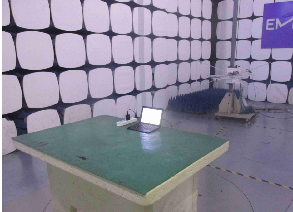
Photograph 2: Set-up for Spurious Emissions for 1 - 18GHz
